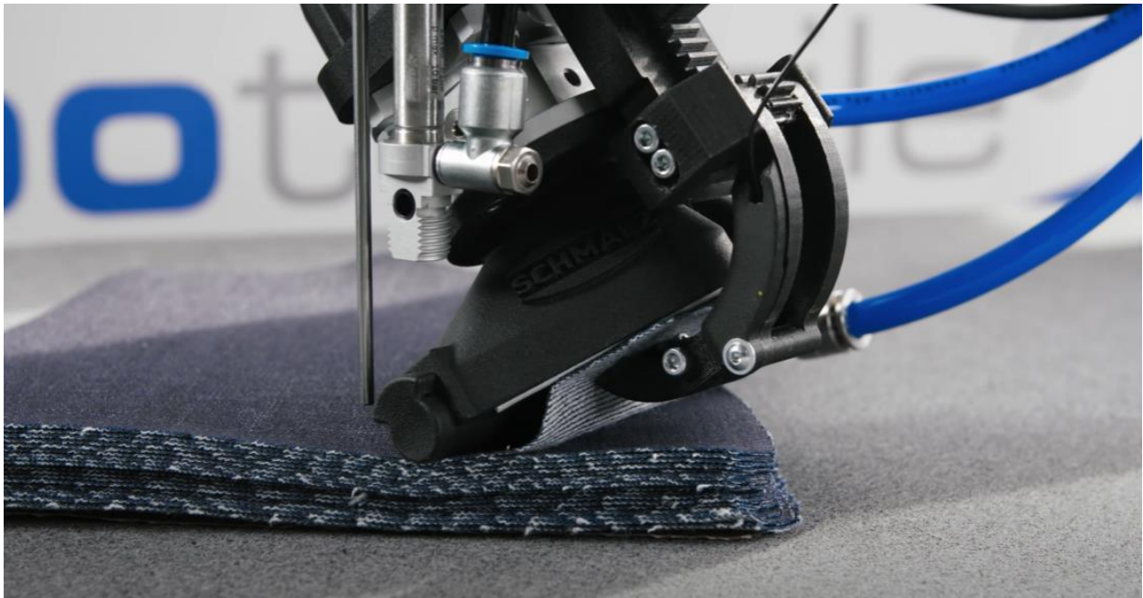
▼ Figure 19 Picture of the gripping principle combination solution of Robotextile (source Robotextile.de)
