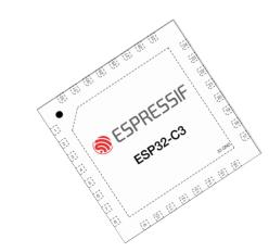
Microcontroller handling local motor control, real-time sensor data acquisition and wireless communication.
